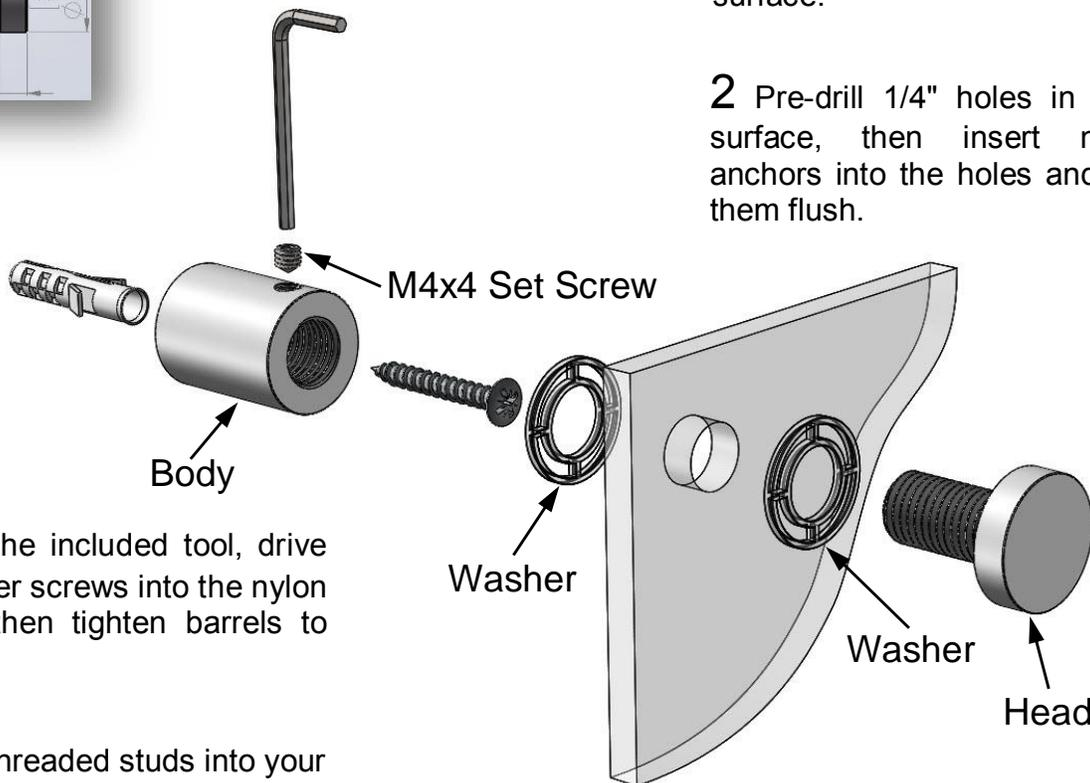
**3** Using the included tool, drive your hanger screws into the nylon anchors, then tighten barrels to surface.
