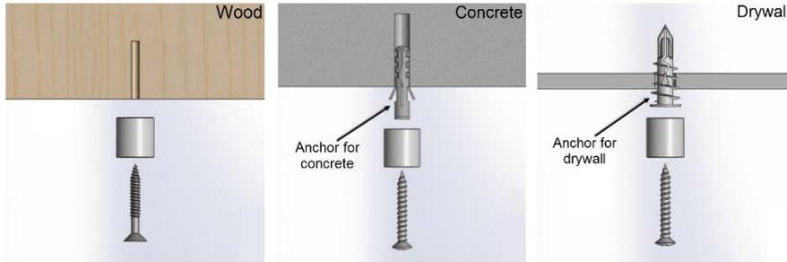
It is essential to check that the top ceiling fixings are strong enough to take the weight of the items being displayed, while allowing for the tension in the cables.. All installation must be done so with proper hardware and protective gears to ensure safety. It is important to check that parts are properly tightened at the end of each installation.
